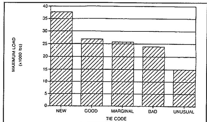
Figure 1 — Maximum static bending load for 20-year-old ties (1).
