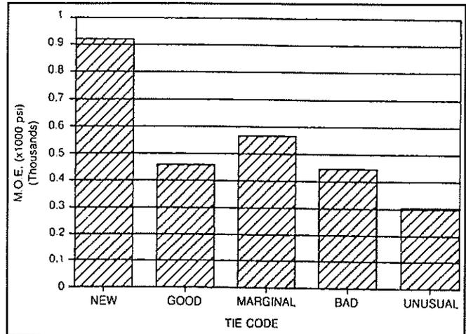
Figure 2 — Bending modulus of elasticity values for 20-year-old ties (2).
